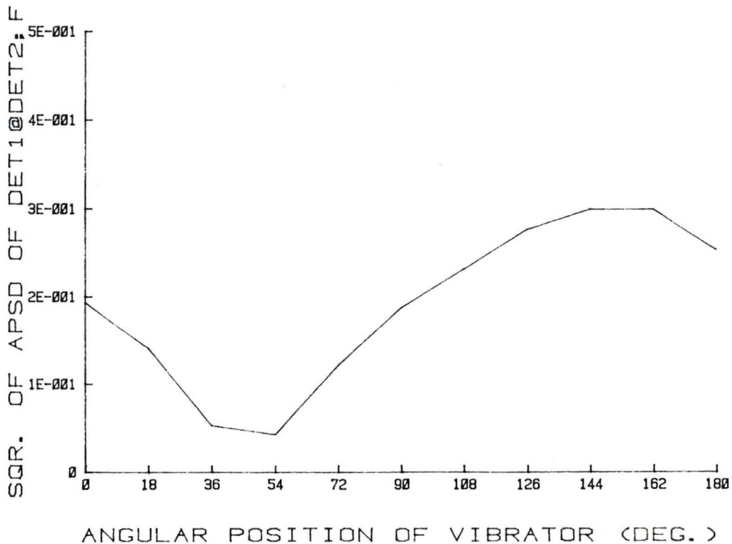
FIGURE 43. Magnitude of DET1 (@DET2) at 1.52 Hz vs angular position of the vibrator (flooded case)
