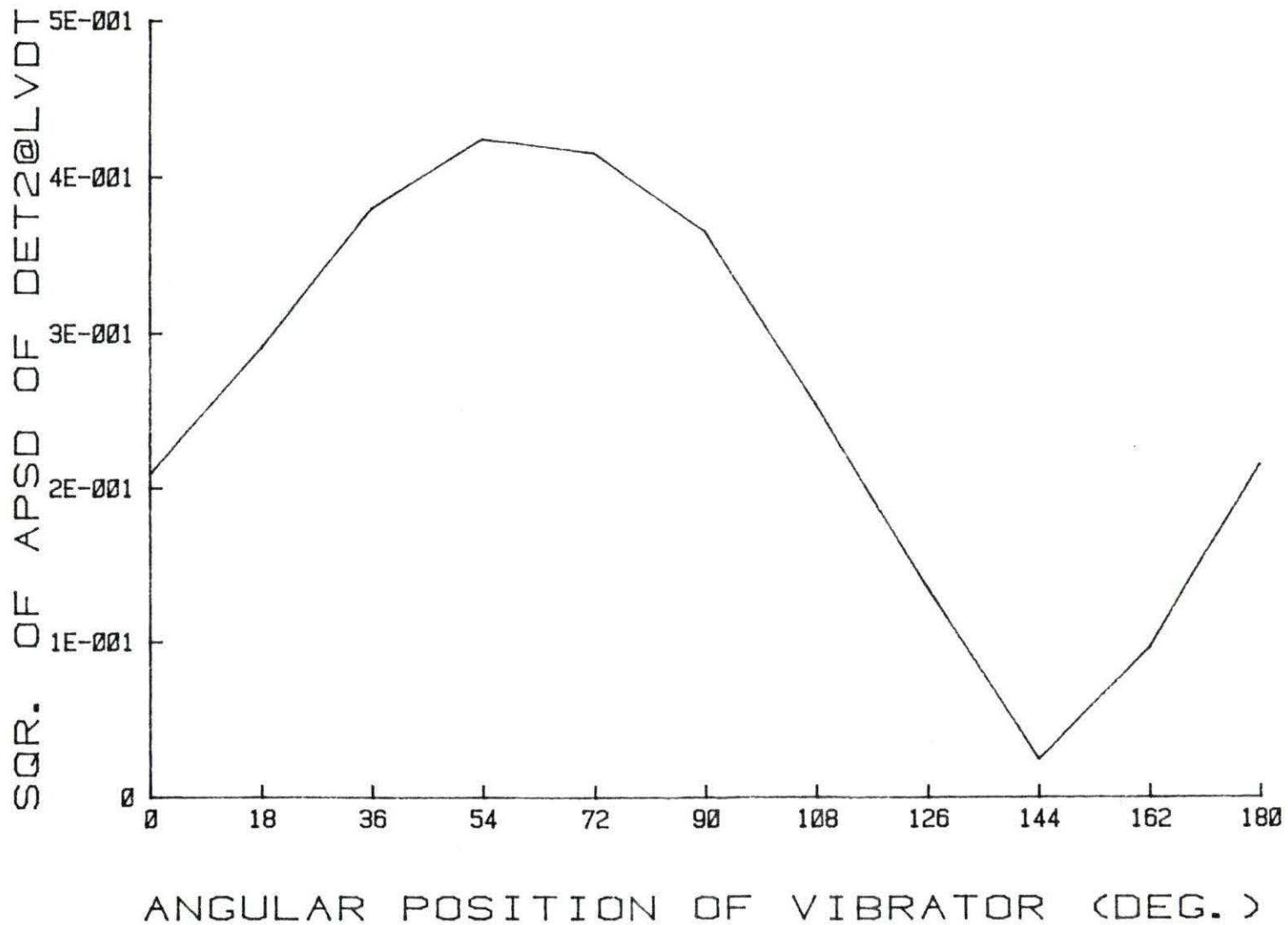
FIGURE 24. Magnitude of DET2 (@LVDT) at 1.52 Hz vs angular position of the vibrator
