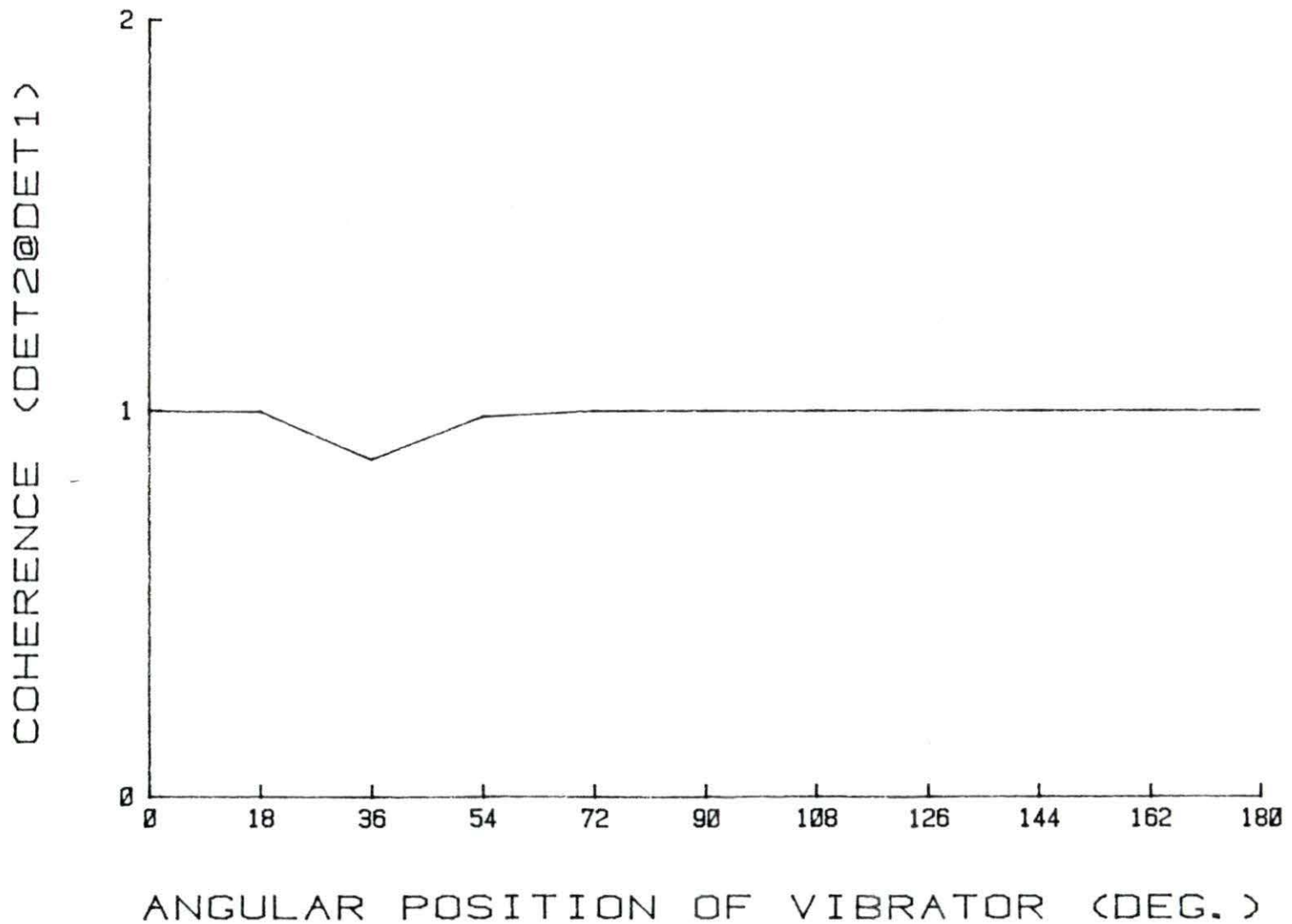
FIGURE 31. DET1-DET2 coherence at 1.52 Hz vs angular position of the vibrator
